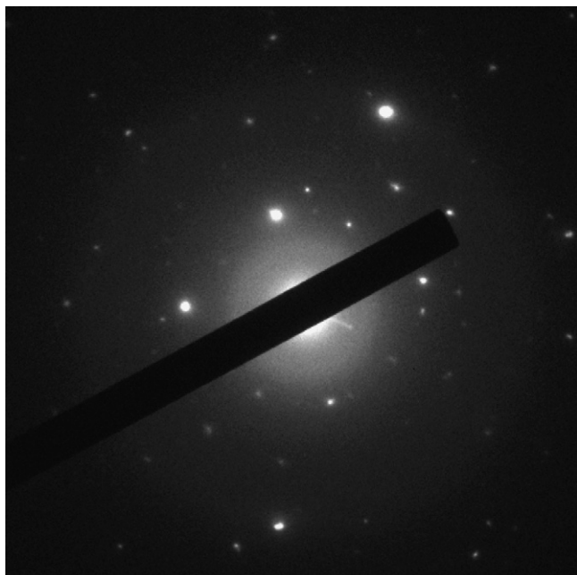
Fig. 8. Selected area diffractions (SAD) image has been obtained from camera lens number 30 on hematite particle that have been shown in Fig. 5 (sample with NaF fired at 900 °C/3 h).
